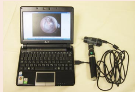
Fig 4: Digital macroview otoscope connected to my laptop
